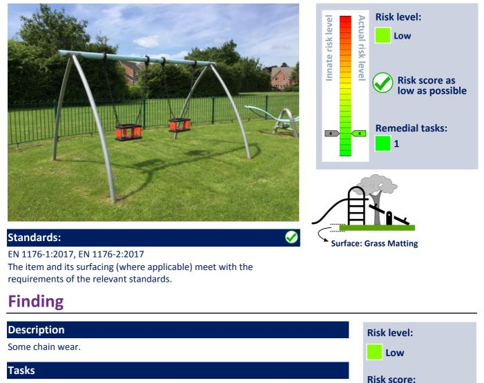
Monitor for further deterioration and replace before 40% wear.
