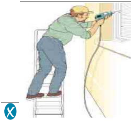
Incorrect – steps side on to work activity
